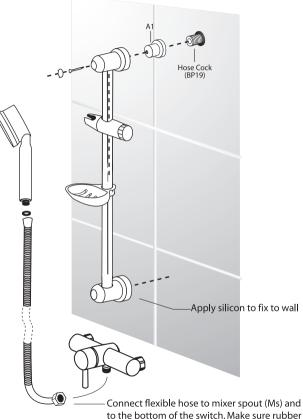
to the bottom of the switch. Make sure rubl washer is in between each connection.
